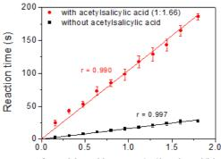
Fig. 1. The calibration curves for ascorbic acid with and without acetylsalicylic acid in a preestablished ratio of 1:1.66
